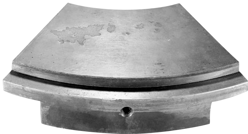
Figure 3. Tin Oxide Damage
