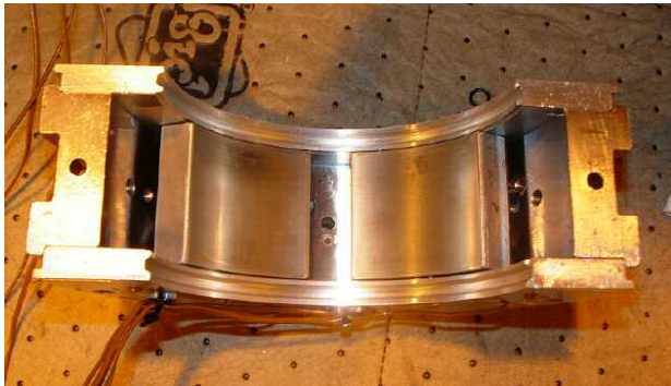
Figure 8. Conventional Bearing with Labyrinth End Seals.
