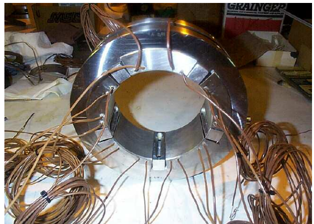
Figure 11. Direct Lube Between-Pad-Groove, Evacuated Configuration.
