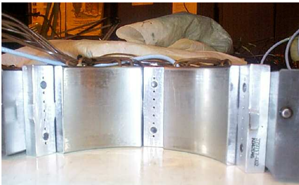
Figure 9. Direct Lube Spray Nozzles, Evacuated Configuration.
