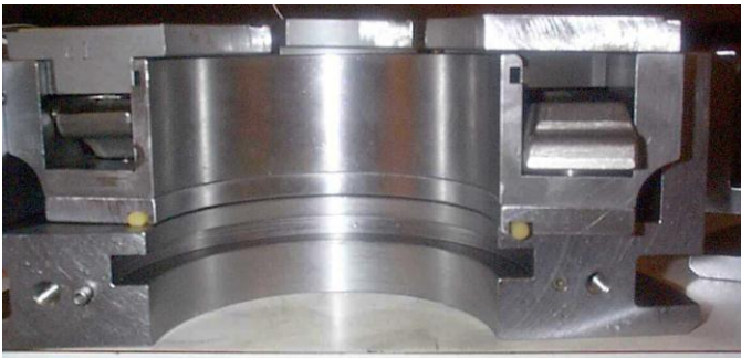
Figure 19: Half Bearing Showing the O-Ring Design.
