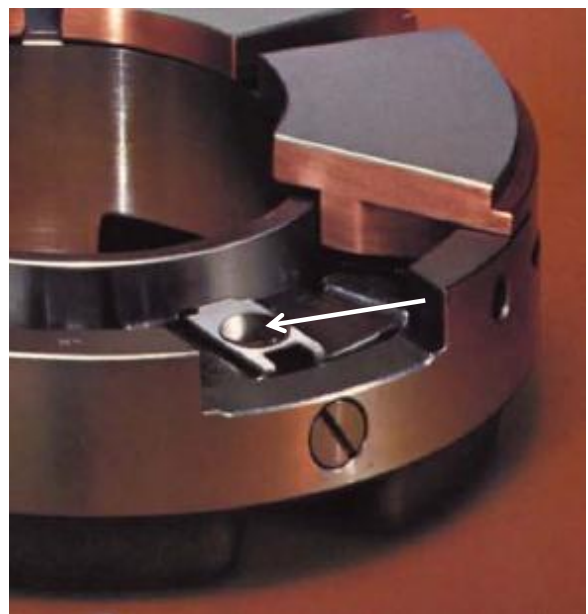
Figure 14: Example Load Cell Position (Thrust Pad Removed).
