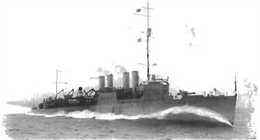
Four-stack destroyer, one of 260 built in World War I for U. S. Navy. Kingsbury Thrust Bearings were used in the turbines, also in the reduction gears to take the propeller thrust.
