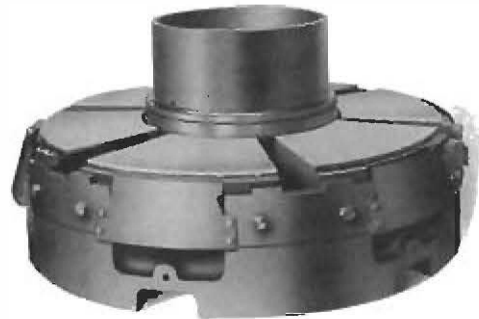
Hydroelectric thrust bearing, equalizing type. For Elliott generator, All-American Canal, California. Size 53 in. Load 555,000 lbs. Speed 150 r.p.m.
