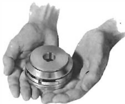
Figure 46 Small one-way three-shoe thrust bearing for airplane supercharger. Load, 1000 lbs.; speed 30,000 r.p.m.
