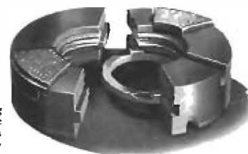
Figure 20 Small two-shoe equalizing bearing for light loads. The split base ring rocks on a blunt knife-edge at right angles to the shoes.
