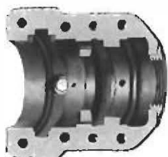
Figure 38 Oil circulator as used in boiler feed pumps.
