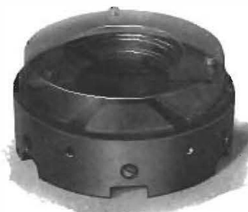
Right—Figure 22 Style KV (6-shoe) thrust bearing for vertical shaft. Runner is shown in phantom. The base ring is in one piece and has a raised shoe-retaining flange. Styles LV and KV have interchangeable dimensions.
