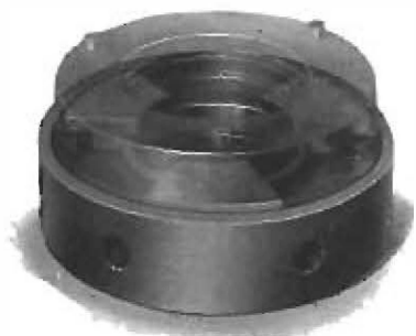
Left—Figure 21 Style LV (3-shoe) thrust bearing for vertical shaft. Runner is shown in phantom. For vertical uses this is often the most convenient form of three-shoe bearing, as it does not require a separate shoe-retaining flange.
